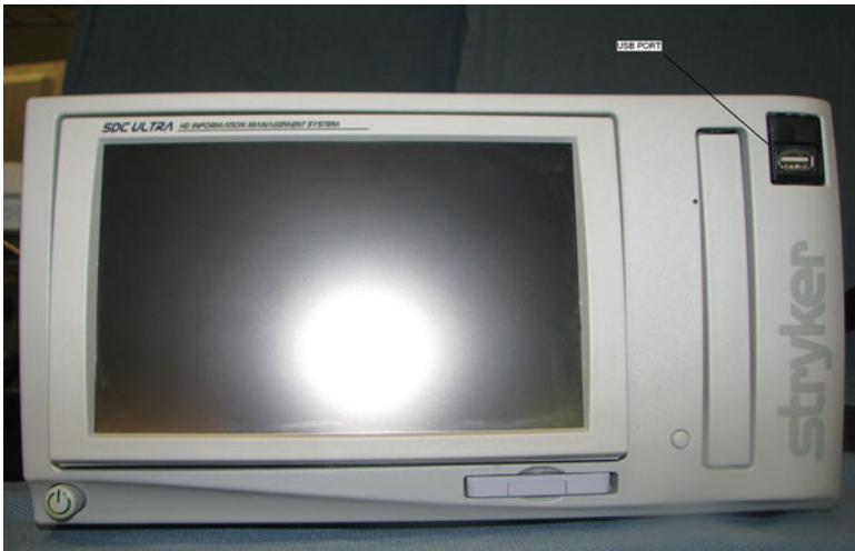
Fig. 13.8. Video capture and storage system capable of exporting images to CD, DVD, and USB devices.
