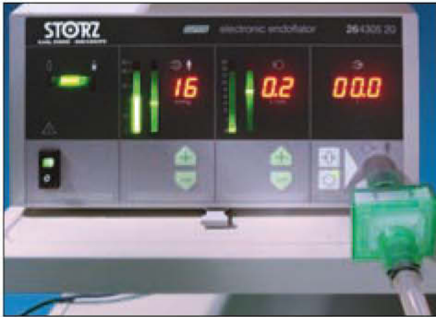
Fig. 11 The intraabdominal insufflation pressure shown on the front panel of the ELECTRONIC ENDOFLATOR® is inappropriate .
