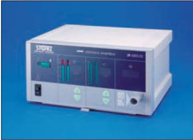
Fig. 13 The CO 2 insufflation unit ELECTRONIC ENDOFLATOR®, (KARL STORZ Tuttlingen, Germany).
