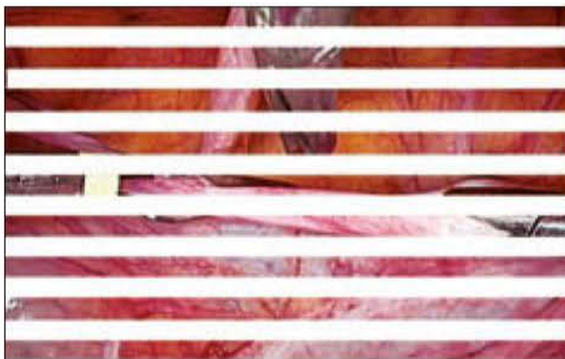
Fig. 35b Interlaced scan (half-frame) displays 25/30* frames per second.
