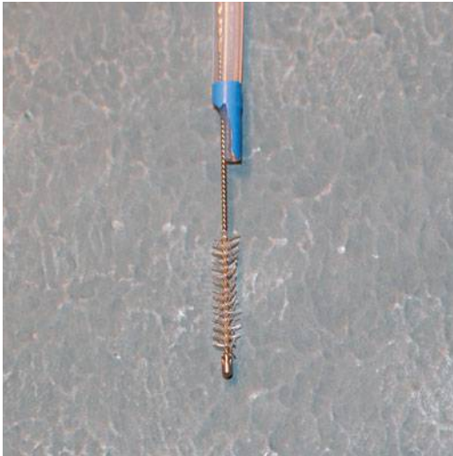
Fig. 2.18. An endoscopic brush that can be placed across a lesion of interest for recovery of a cellular sample.
