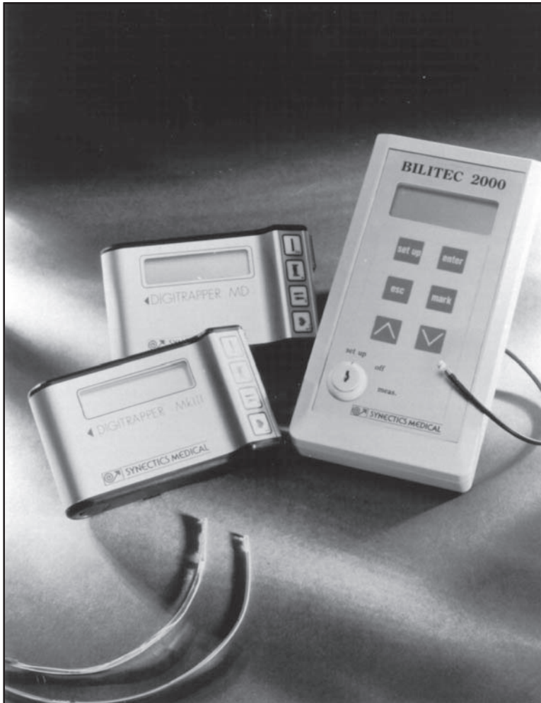
Figure 8.1. These are data loggers used for ambulatory pH monitoring. Also pictured are two pH probes (photograph courtesy of Medtronic Synectics).
